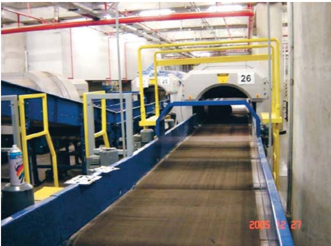
Searching using In-line Screening system and CTX
