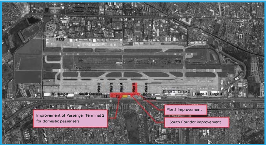
Short-term and urgent development plan under Don Mueang International Airport Development Project Phase 2 (2013 - 2014)
